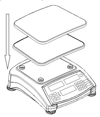
Figure 2-1. Installing sub-platform and metal pan
