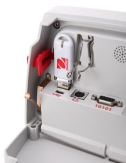
Interface connections inside of the Terminal.
